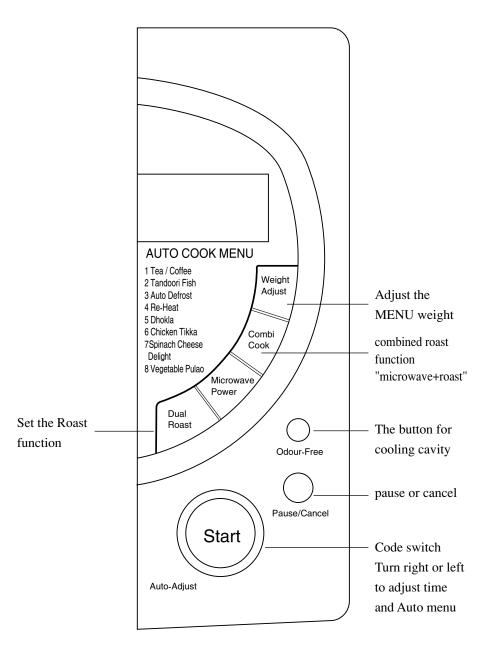
This model of microwave oven offers four different design of usage according to the demand of the users: I. Microwave only; II. Double-side roast; III. Combination of the microwave and double-side roast; IV. Auto-menu. Details as per following: I Use the microwave only.
